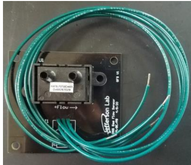
Gas Flow Sensor board with test leads.
